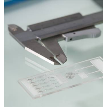
Physio Check - passive Lab-on-a-chip-system for diagnostics
